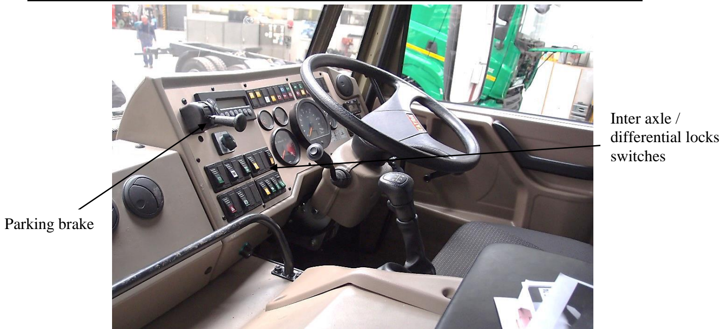
Fig 2: Controls of Pneumatic System in panel board
